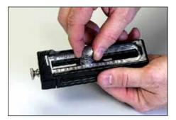
Remove top nut and pivot post from cutter block.
