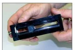
To cut a desired width, set indicator to double the width plus 3/16". For example, to cut a 1/2" width, set indicator to 1 3/16".
