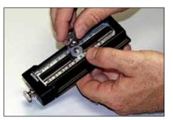
2. Place post washer on pivot post and reinstall pivot post into cutter block with flat side of pivot post facing cutting blade. Reinstall top nut.
