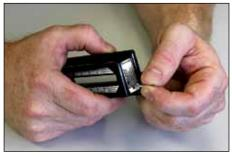
2. Use the appropriate length center pin for the thickness of material being cut. Insert center pin in silver encircled hole in the end of the cutting block.
