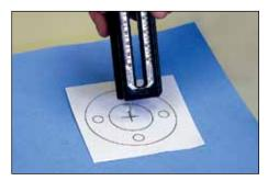
Using cutter block as a handle, pierce center of gasket with center pin. Remove the cutter block and center pin will remain in gasket material.
