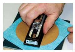
Place template with disc pivot pin on gasket material and push disc pivot pin into gasket to make an indentation.
