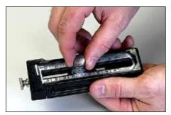
6. Loosen top nut and adjust pivot post to desired cutting diameter by matching pivot post indicator line with appropriate dimension of 0"- 6" scale. Secure with top nut.
