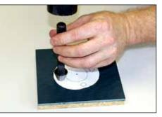
**10.** Reset cutter block for bolt holes and cut, or use hole punches to create bolt holes.
