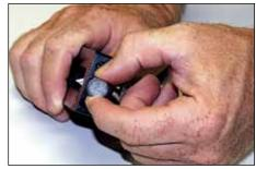
Loosen thumb screw of cutter block and position cutting blade so it protrudes slightly beyond thickness of gasket material. Tighten thumb screw.
